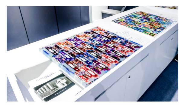
In the demonstration using transparent film, four colors were printed first, followed by interdeck drying and then white ink printing. The demonstration showed how stable paper feeding and delivery performance can be maintained even with special substrates, enabling high-quality printing.
