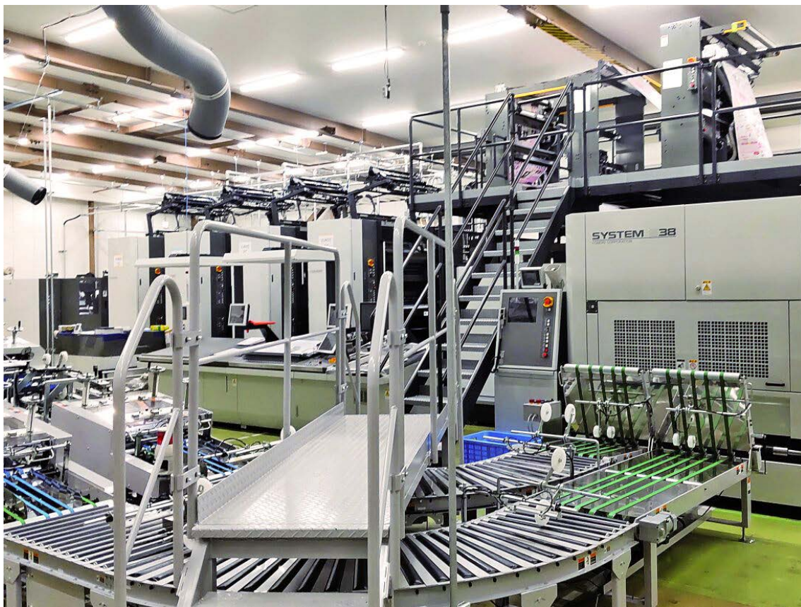
In-line folder equipped on the System G38
